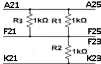
Figure 1.5 Resistor Schematic with Console Breadboard Connection Points Indicated
