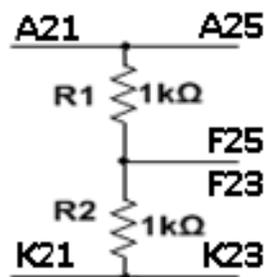
Figure 1.4 Two Resistor Schematic with Console Breadboard Connection Points Indicated
