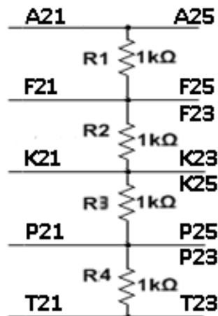
Figure 1.6 Four Resistor Series Circuit with Console Breadboard Connection Points Indicated
