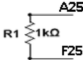
Figure 1.3 One Resistor Circuit Schematic with Console Breadboard Connection Points Indicated
