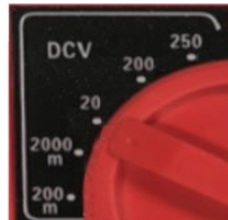
Figure 1.9 CenTech Meter – Volts Ranges (set at 20 volts)
