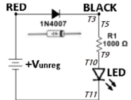
Figure 2.3. Forward Biased Diode
