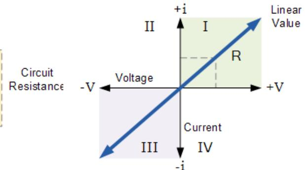
Fig 2.6 I-V Curve for a Resistor
