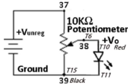
Figure 2.2. Variable Power Source and LED
