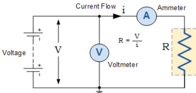
Fig 2.5 Characteristic Curve Measuring Circuit
