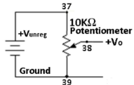
Figure 2.1. Variable Power Supply
