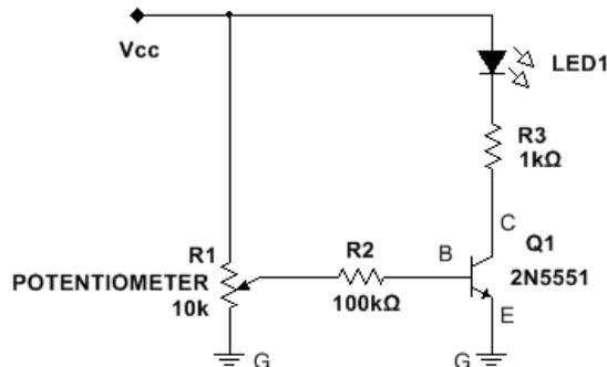
**3.3.b)** Using the **10Kohm** pot knob to adjust the voltage available to the 100K resistor in the transistor's base circuit it should be possible to vary the brightness of the LED in the collector circuit. Did this work ? ( \_\_\_ YES \_\_\_ NO )
