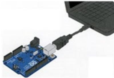
**Figure 3.1. Attaching the Arduino**
