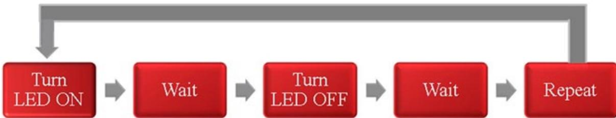
*Figure 3.9. Flow Chart for Arduino-controlled LED*
