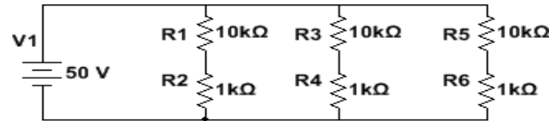
Figure 6.1 Series-Parallel Resistor Circuit
