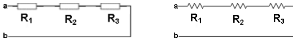
Figure 1.8 Pictorial Diagram and Schematic for Series Circuit
